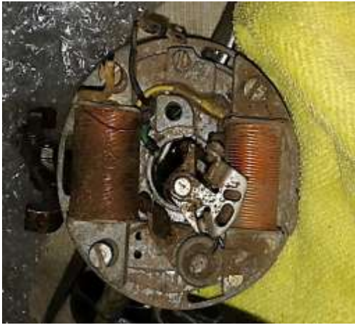
Condition of original magneto
