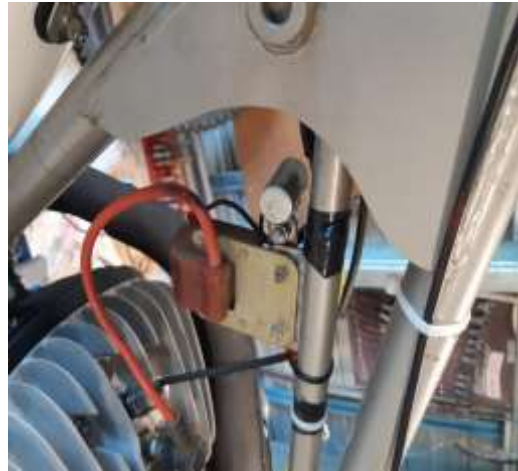
Condenser relocated to frame tube
