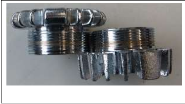
750 nut with longer thread on the top, 850 with shorter on right.
